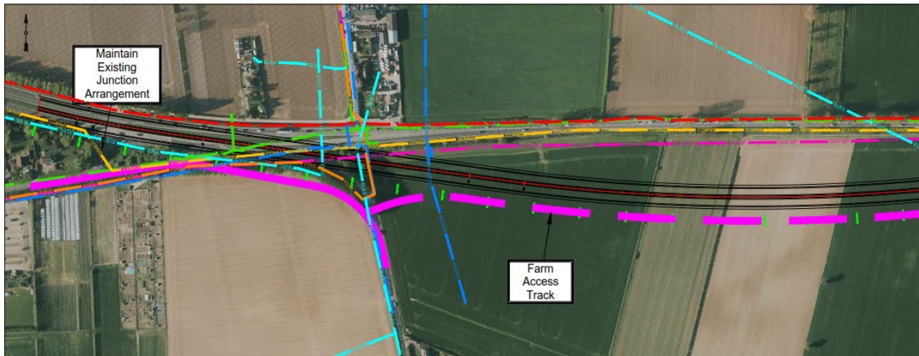
Figure 4-5: Yarmouth Road Junction arrangement, Option E
