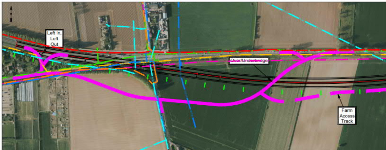
Figure 4-1: Yarmouth Road Junction left in, left out arrangement, Option A
