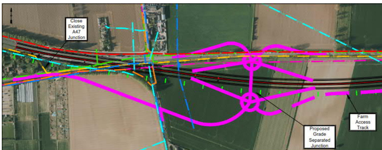
Figure 4-2: Yarmouth Road Junction arrangement, Option B
