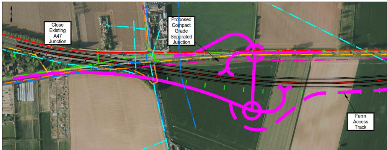
Figure 4-3: Yarmouth Road Junction arrangement, Option C
