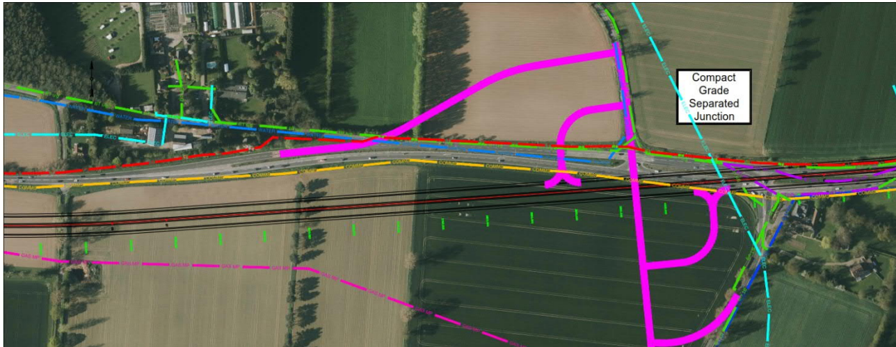
Figure 4-10: B1140 Junction arrangement, Option E
